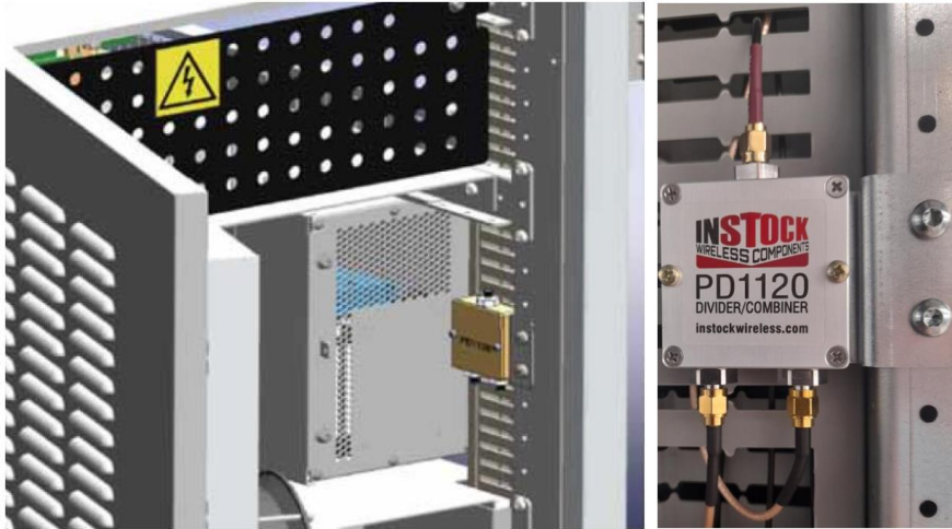
Figure 7 Location of signal splitter
