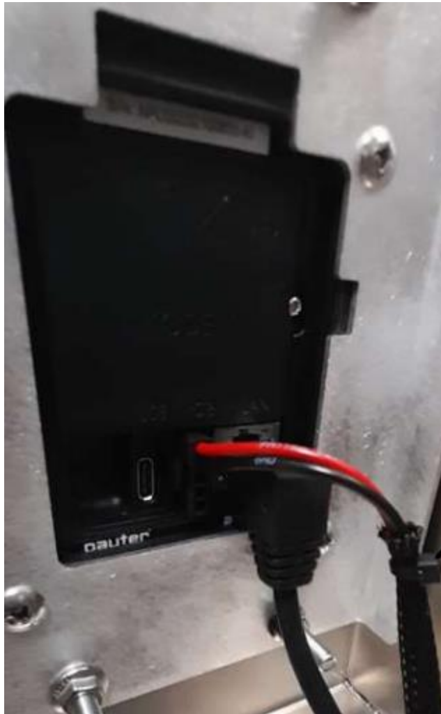
Figure 10 New routing of antenna cable to Payter terminal (left to right)
